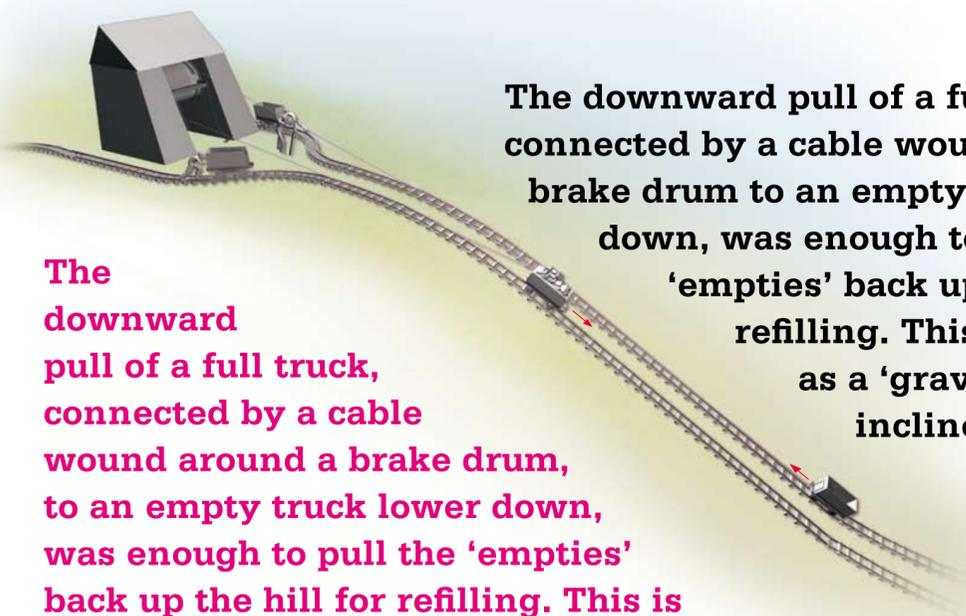
The downward pull of a full truck, connected by a cable wound around a brake drum to an empty truck lower down, was enough to pull the 'empties' back up the hill for refilling. This is known as a 'gravity balanced' incline.
